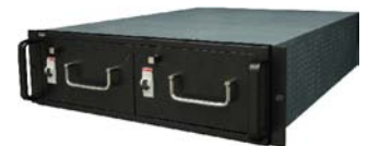
Battery Module with 20pcs 12V/9AH
